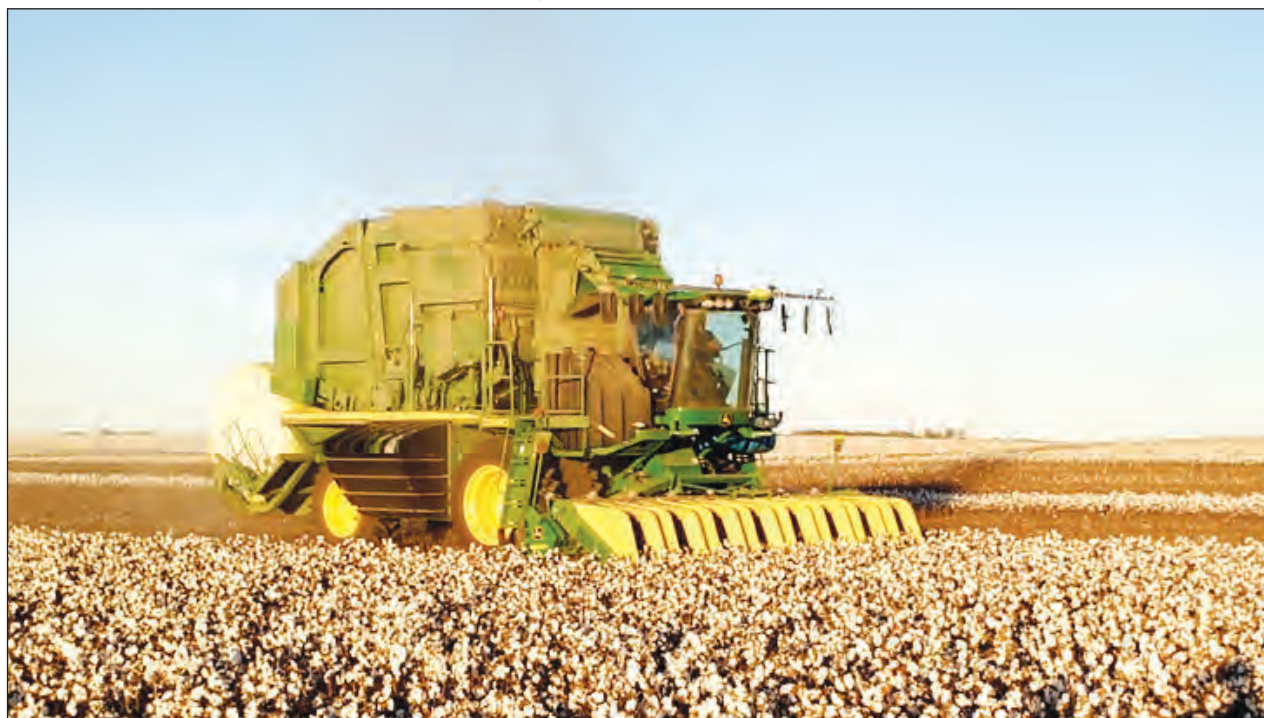
Bale strippers allow one operator to harvest and roll the cotton into big round bales ready to be taken to the gin.
