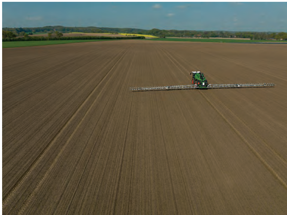
Pictured is a Fendt Rogator 665 using the Smart Spraying Solution targeted spraying in a green-on-brown trial application. Photo courtesy of Business Wire
