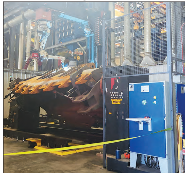
Robotic welders are also utilized in the manufacturing process at Work Tools.
