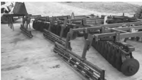
25' Krause 4900 fitted with rolling harrow.
