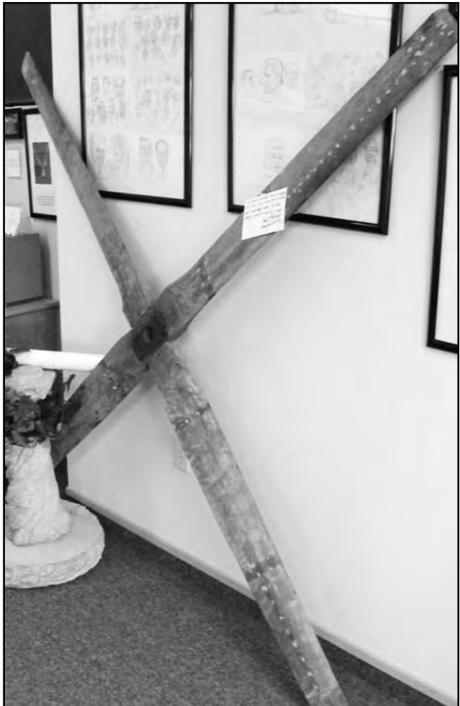
Hand-carved by Boyer's father, this propeller was part of a wind charger that made their home one of the first in Republic County to have electricity.
