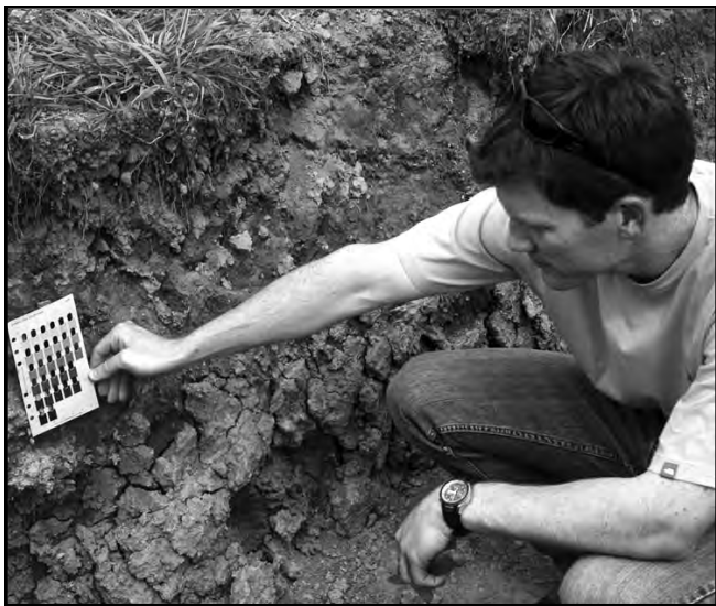
O'Donnell places a page from a set of Munsell soil color charts against exposed soil at MU South Farm.
