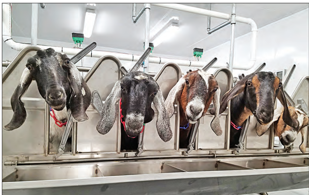
The goats are milked on a raised stanchion that will accommodate six at a time and includes a closed pipe milking system and automatic clean and sanitize device.
