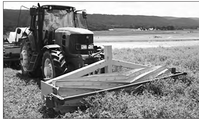
Farmers roll a hairy vetch-triticale cover crop into a thick mat which serves as a mulch and weed-suppressant.
