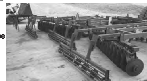
25' Krause 4900 fitted with rolling harrow.
