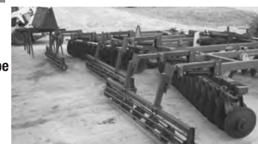
25' Krause 4900 fitted with rolling harrow.
