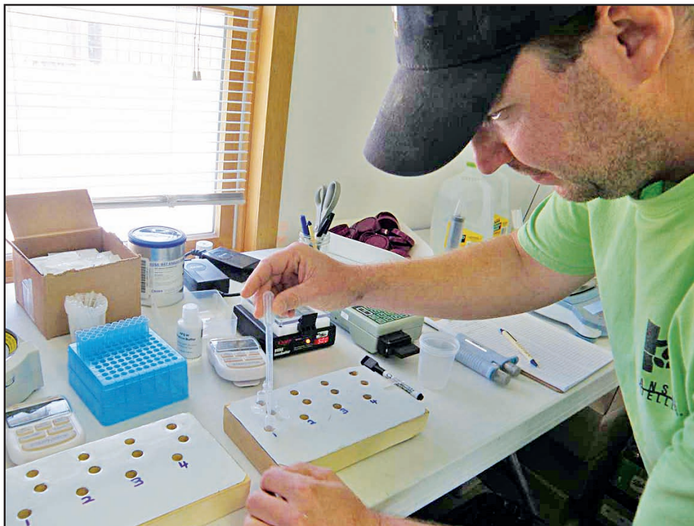
Hansen-Mueller employee Clint Strait demonstrates the lab work to test for aflatoxin in trucks hauling corn.
