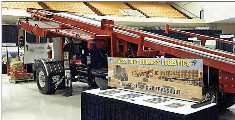
The Stinger Bale Stacker was on display at the Kansas Energy Conference Trade Show. It can stack large square bales of biomass feedstock for storage or roadside them for transport.
