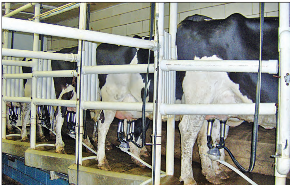
An innovation on AndyAcres dairy farm was replacing the traditional steel pipe milk stanchions with PVC pipe in 1996. He milks 60 Holsteins and has five PVC stanchions on each side for a total of 10 milking cows at a time. According to dairyman Doug Anderson, the main advantage of PVC pipe is low maintenance because they don't rust and they are easy to clean.
