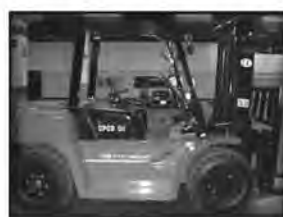
YTO CPCD50 forklift 11,023lbs lift capacity
